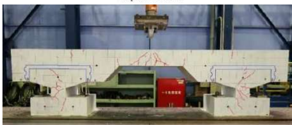
Figure-6 Full-scale structural performance verification experiment (load transfer verification)
