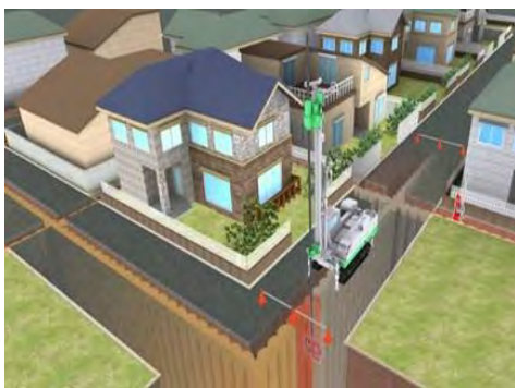
Fig.1 Surround Housing Plot with Improved Soil Wall
