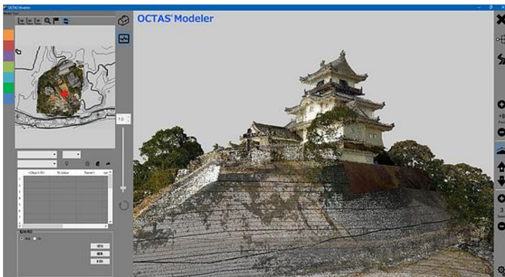
Figure 6: An example of a walkthrough display of ground laser point group data
