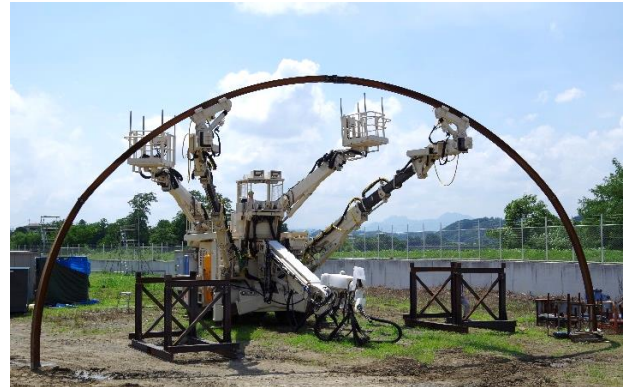
Photo-1 Steel Timbering Erecting Robot
