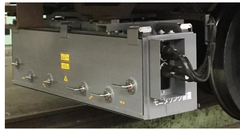
Photo1 Track geometry measurement device
