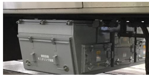
Photo2 Track material monitoring device
