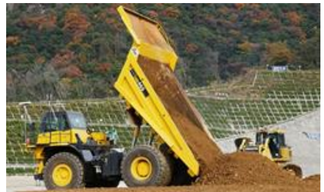
Fig. 5 The cooperative work of automated dump truck and bulldozer
