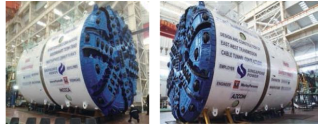
Photo 1 Mud pressure shield
