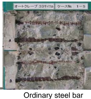
Photo 1 Corrosion of reinforcement after accelerated test (Equivalent to 100 years' service life)
