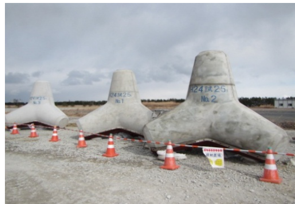
Photo 2 Wave dissipating concrete block using sea water
