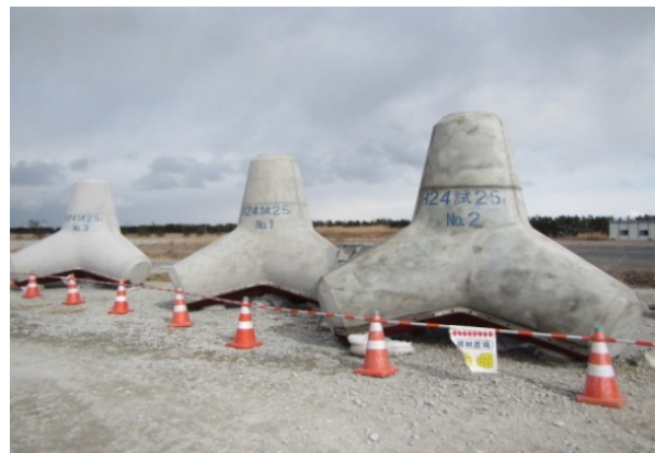
Photo 2 Wave dissipating concrete block using sea water
